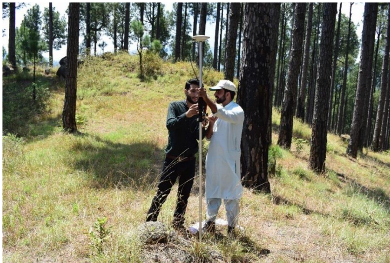
Figure 23 DGPS rover station on top of an unmarked forest boundary in Manshera, KP
