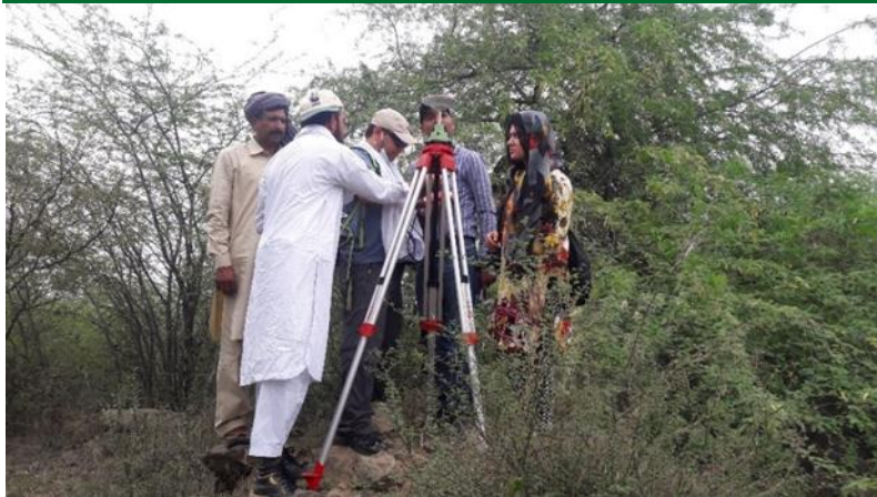
Figure 22 DGPS base station being established in one of the forest boundary pillars (Jhelum, PB).
