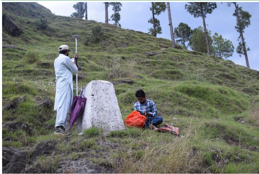
Figure 24 DGPS rover station being established in a forest boundary in pillar Manshera, KP.
